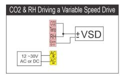
In this example the CO2 and RH is controlling the VSD with a high select. Both the CO2 and RH outputs are individually scalable so the CO2 range can be 450ppm to 1,000ppm and the RH range can be 75% to 100%. Also, the RH output can be limited to 7V max if required.
