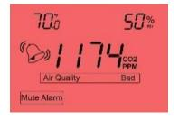
When enabled, user can mute an audible alarm by pressing the "Mute Alarm" button when shown. If Active Ventilation is enabled, the user can tap the "A" icon to briefly display the outside air temperature.
