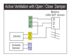
In the Installer menu you must activate the Active Ventilation function by setting the inside and outside air temperature thresholds (page 6 explains this) and defining the active ventilation output options. Once you have completed these three steps the letter "A" will be shown the in the lower right corner of the LCD to confirm the Active Ventilation function is active.
