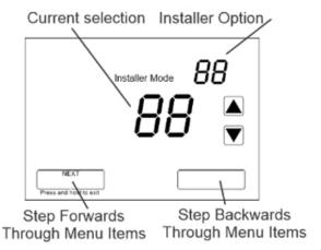
Use the Up (or Down) arrow to adjust the display to "21" (twenty-one) or your previously saved PIN. Press the NEXT button to enter the menu. If you are returned to the previous screen, you have entered the incorrect PIN. Try again.
