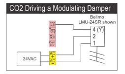
Whether you wish to control a Variable Speed Drive or a modulating damper the wiring and setup are the same. You can also mix the devices you wish to control with the three 0-10V outputs. All three outputs can be individually scaled.
