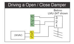
An open/close or an off/on output can be controlled by the monitor using the volt free relay provided. The relay threshold can be individually adjusted for each sensor. (30V @ 1A max)
