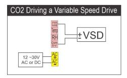
In this example a standard Variable Speed Drive is being controlled with the CO2 0-10V output. The Installer menu permits you to scale the 0-10V output to match your requirements such as output 0V at 450ppm and output 10V at 800ppm.
