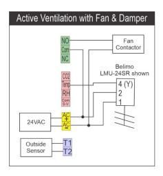
If you would like, you can have both the temperature 0-10V output and volt free relay used for advanced ventilation. In the Active Ventilation Output options menu settings select both relay and temp 0-10 (option 3). This permits you to open the fresh air damper and turn a fan on for example if outside air is suitable.
