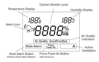
When enabled, the user can press the "Force Fresh Air" button which will bring in fresh air. The "Force Fresh Air" button will flash when pressed to indicate that it is running. When enabled, the LCD backlight can also change the background color from green, amber, and red to visually indicate the CO2 level in the space.
